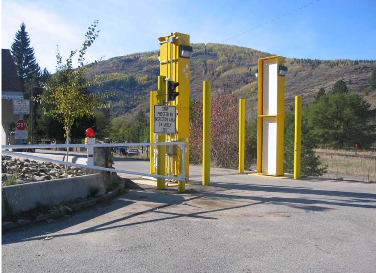
Figure 7 - A radiation portal monitor, such as installed at many roadway points of entry into the United States. The devices are used to scan entering vehicles and cargo for radioactive materials. (Photograph courtesy of the Pacific Northwest National Laboratory)
