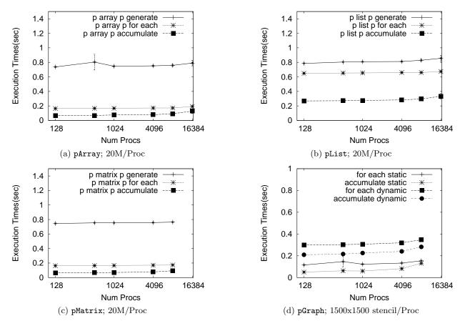
Figure 4: Execution times for p\_for\_each, p\_generate, p\_accumulate algorithms on CRAY for different data structures. (a) pArray with 20M elements per processor, (b) pList with 20M elements per processor, (c) pMatrix with 20M elements per processor, and (d) pGraph with 2.25M elements (1500x1500 stencil) per processor.
