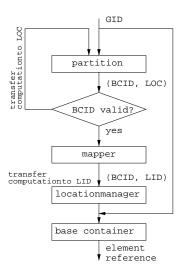
Figure 2: pContainer modules interaction to find the element reference corresponding to a given GID.
