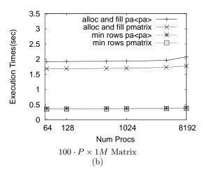
Figure 8: Comparison of parray > (pa<pa>) and pMatrix on computing the minimum value for each row of a matrix. Weak scaling experiment with (a)  $P \times 100M$  and (b)  $100 \cdot P \times 1M$  elements. parray > takes longer to initialize while the algorithm executions are similar.
