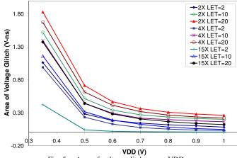
Fig. 5. Area of voltage glitch versus VDD
