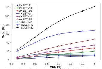
Fig. 4. Charge collected at the output of INV for different values
