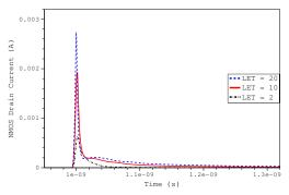
Fig. 3. Radiation induced drain current of the NMOS transistor of  $4\times$  INV with VDD=1V
