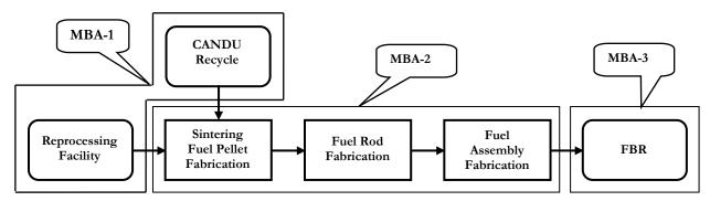
Figure 1. Schematic of Material Balance Areas for Fuel Fabrication Facility
