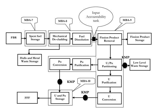
Figure 4. Schematic of the Material Balance Areas for the Fast Reactor Fuel Reprocessing
