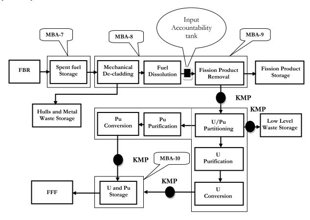
Figure 6. Schematic of MBAs for the FRFRF using PRAETOR Risk Informed Safeguards
