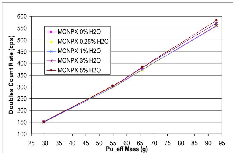
Figure 5. Double rates vs.  $Pu_{eff}$  for various water contents.
