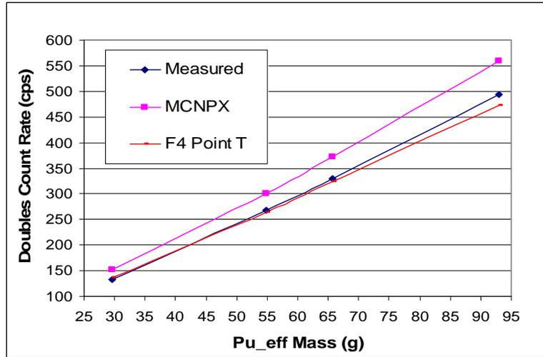
Figure 4. Doubles rate as a function of  $Pu_{eff}$  mass.
