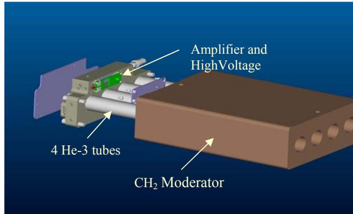
Figure 1. Individual slab of PNCC.
