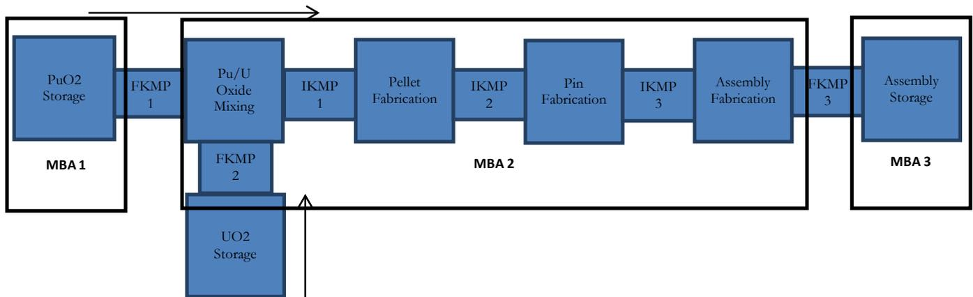
Fig. 3: MBA plan for the fuel fabrication facility.
