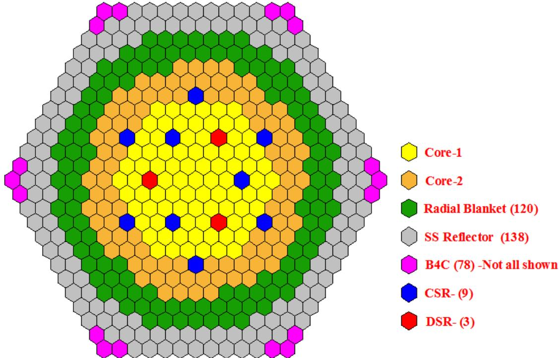
Fig. 1. Core configuration for 500MWe PFBR-style reactor.<sup>2</sup>
