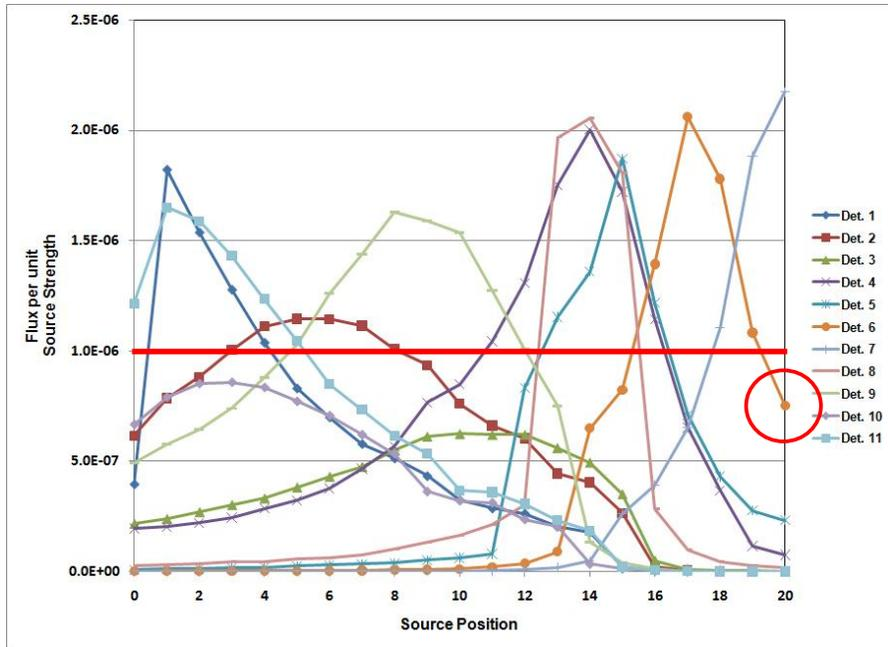
**Figure 3.** Flux per unit Source Strength vs Source Position for 11 detectors
