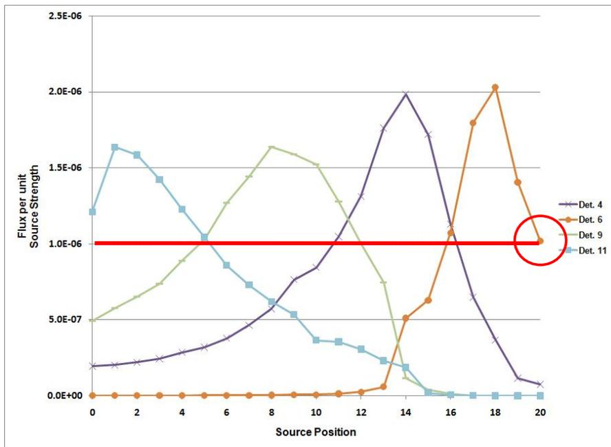
Figure 6. Flux per unit Source Strength vs Source Position for Detectors 4, 6 (modified), 9, and 11
