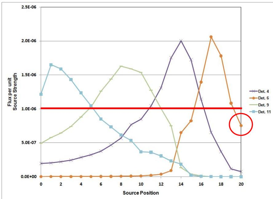
**Figure 4.** Flux per unit Source Strength vs Source Position for Detectors 4, 6, 9, and 11
