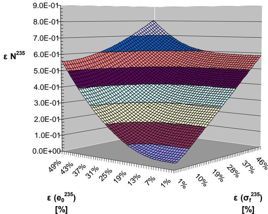
**Figure 2.** Error in the calculated  $^{235}\text{U}/^{238}\text{U}$  value as a function of the error in the  $^{235}\text{U}$  enrichment and the  $^{235}\text{U}$  microscopic fission cross-section.
