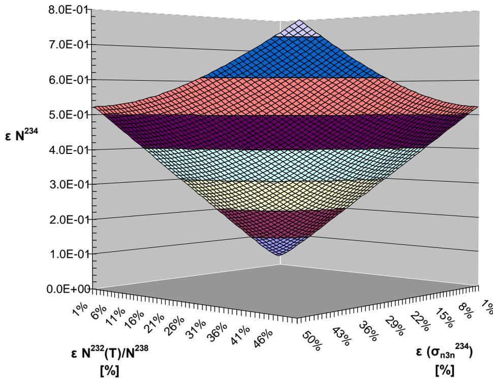
**Figure 1.** Error in the calculated  $^{234}\text{U}/^{238}\text{U}$  value as a function of the error in the measured  $^{232}\text{U}$  value and the  $^{234}\text{U}(n, 3n)$  microscopic cross-section.
