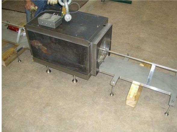
Fig. 3. The iron shielding and fuel pin support structures are depicted.
