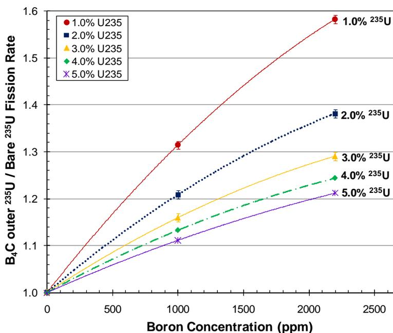
**Figure 4.** Comparison of  $B_4C$  outer  $^{235}U$  FC to bare  $^{235}U$  FC ratio for different  $^{235}U$  enrichments versus boron concentration in water.
