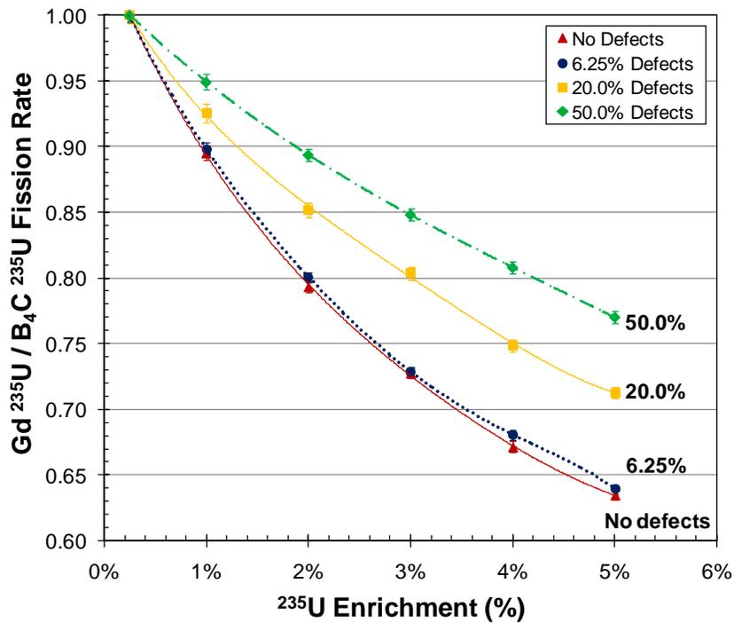
**Figure 6.** Effect of partial defects on ratio of Gd covered <sup>235</sup>U FC to B<sub>4</sub>C outer <sup>235</sup>U FC (epithermal to fast flux ratio) with 2200-ppm boron in *water* versus <sup>235</sup>U enrichment.
