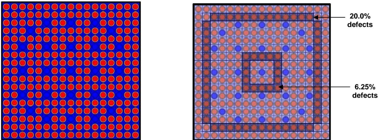
Figure 3. Top view of PWR 17x17 assembly (left) and partial defects locations (right).
