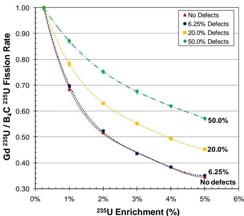
**Figure 7.** Effect of partial defects on ratio of Gd covered  $^{235}\text{U}$  FC to  $\text{B}_4\text{C}$  outer  $^{235}\text{U}$  FC (epithermal to fast flux ratio) in *air* versus  $^{235}\text{U}$  enrichment.
