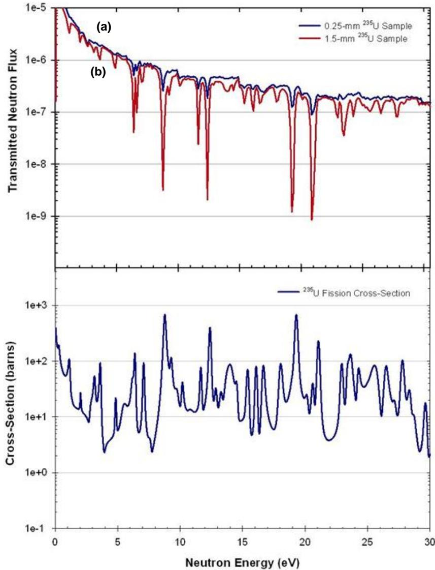
**Figure 1.** Comparison of the absorption lines in the neutron flux after transmission through a 0.114-mm Gd filter and 0.25-mm [curve (a)] and 1.5-mm [curve (b)]  $^{235}\text{U}$  metal sample (upper plot) to the  $^{235}\text{U}$  fission cross-section at neutron energies  $\leq 30$  eV (bottom plot).<sup>2</sup>
