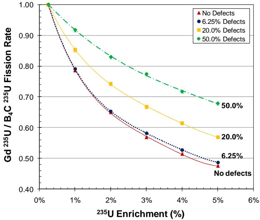
**Figure 5.** Effect of partial defects on ratio of Gd covered <sup>235</sup>U FC to B<sub>4</sub>C outer <sup>235</sup>U FC (epithermal to fast flux ratio) in *water* versus <sup>235</sup>U enrichment.
