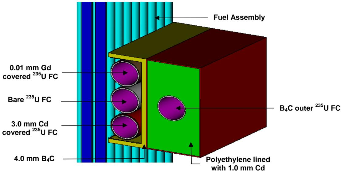
Figure 2. Detector configuration located adjacent to assembly.
