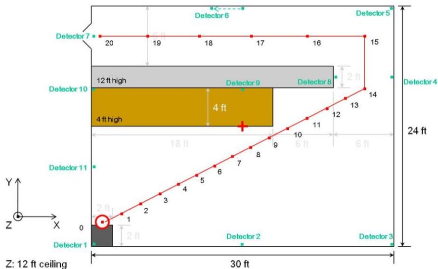
Figure 5. Detector 6 repositioned for 4-detector optimized system
