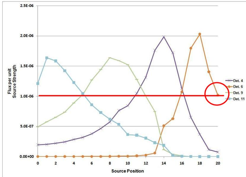
Figure 6. Flux per unit Source Strength vs Source Position for Detectors 4, 6 (modified), 9, and 11
