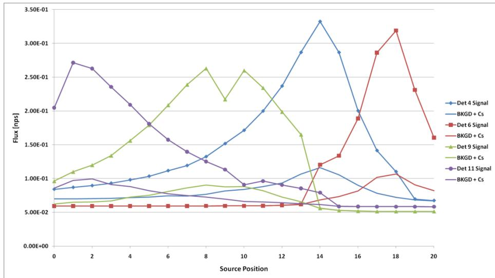
Figure 10. Tracking U with background contributions from  $^{40}\text{K}$  and  $10\text{-}\mu\text{Ci } ^{137}\text{Cs}$  source
