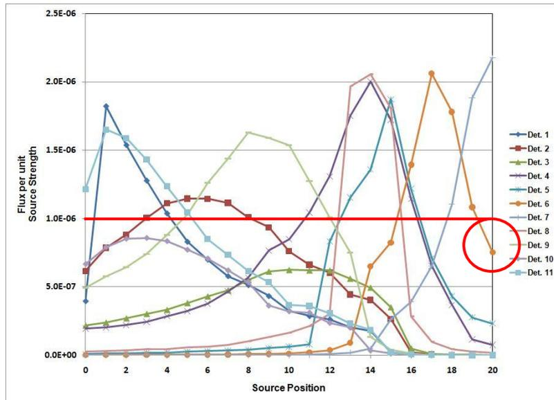
**Figure 3.** Flux per unit Source Strength vs Source Position for 11 detectors
