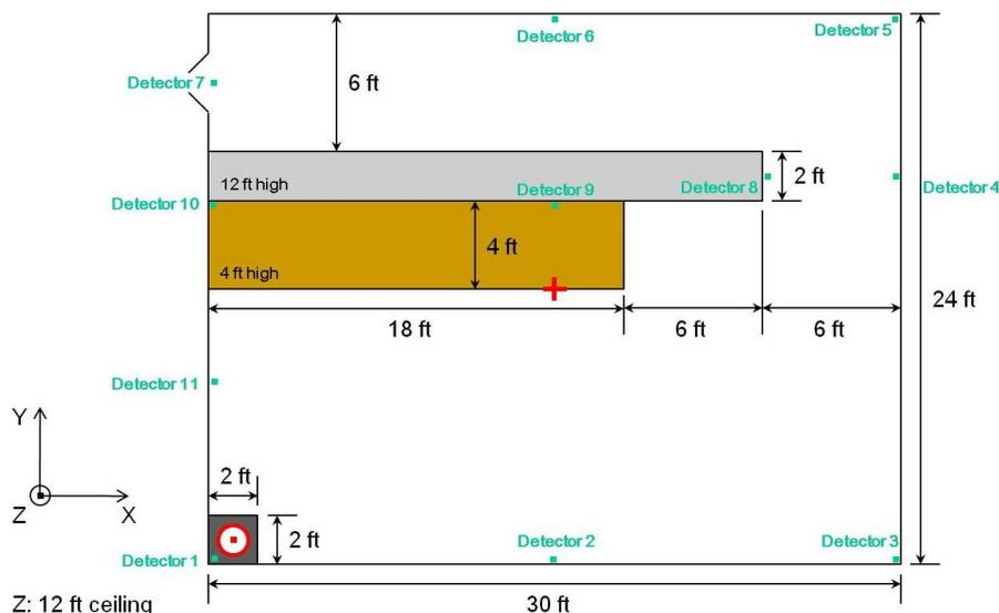
**Figure 1.** TAMU ASTL with source in safe (the red/white target is the source)
