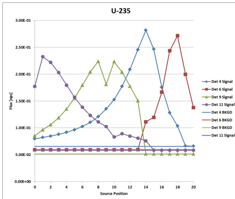
Figure 8. Tracking  $^{235}\text{U}$  with 4 detectors and associated background from  $^{40}\text{K}$
