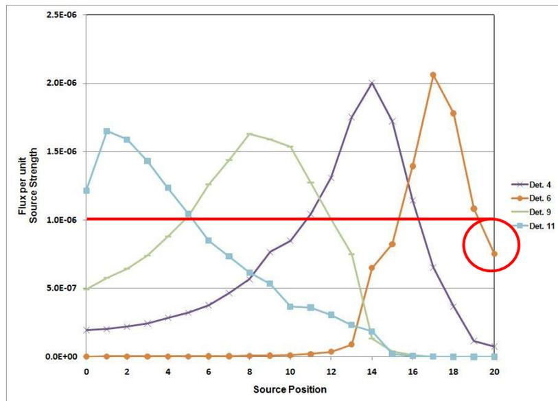
Figure 4. Flux per unit Source Strength vs Source Position for Detectors 4, 6, 9, and 11
