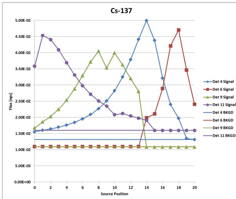
Figure 7. Tracking  $^{137}\text{Cs}$  with 4 detectors and associated background from  $^{40}\text{K}$
